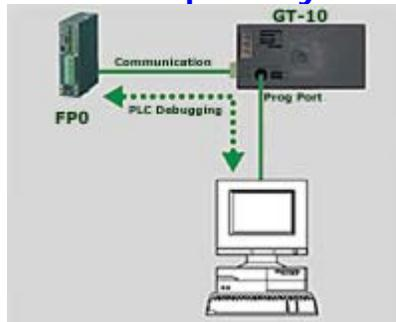
Two RS232C ports are available for connecting to the PLC and the PC. This allows you to program both the PLC and GT-10 without having to unplug any cables. It is also possible to connect a modem to
