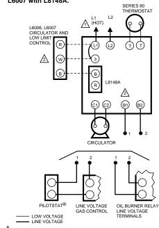
POWER SUPPLY. PROVIDE DISCONNECT MEANS AND OVERLOAD PROTECTION AS REQUIRED.
