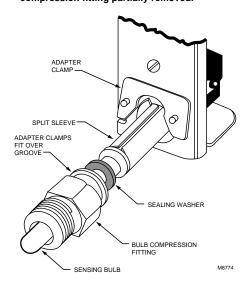
Fig. 4—Mounting L6006C on pipe or tank.
