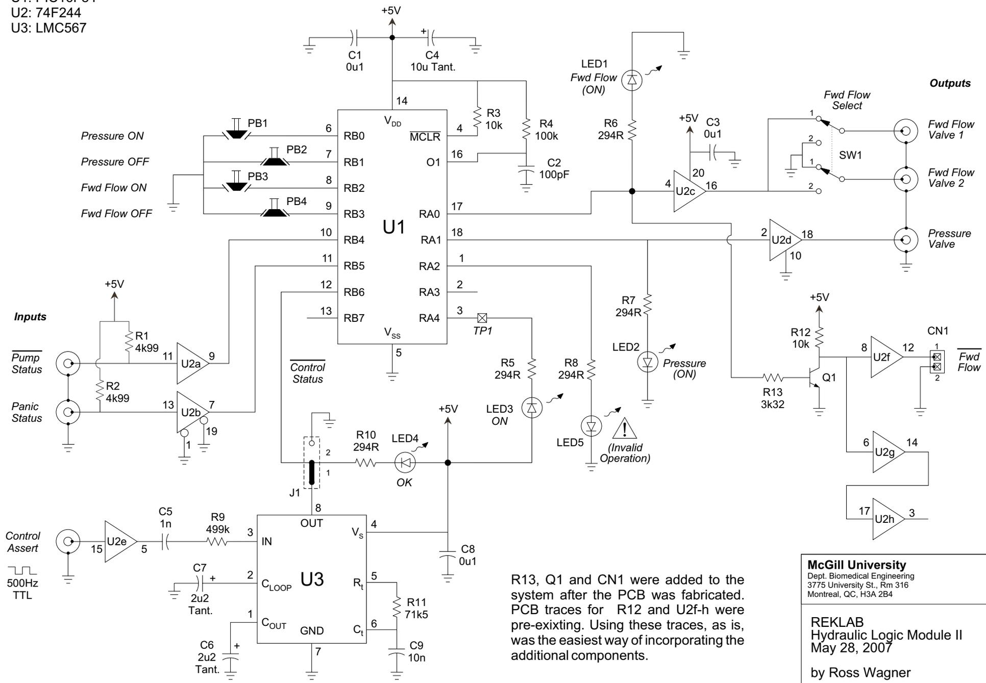
R13, Q1 and CN1 were added to the system after the PCB was fabricated. PCB traces for R12 and U2f-h were pre-existing. Using these traces, as is, was the easiest way of incorporating the additional components.
