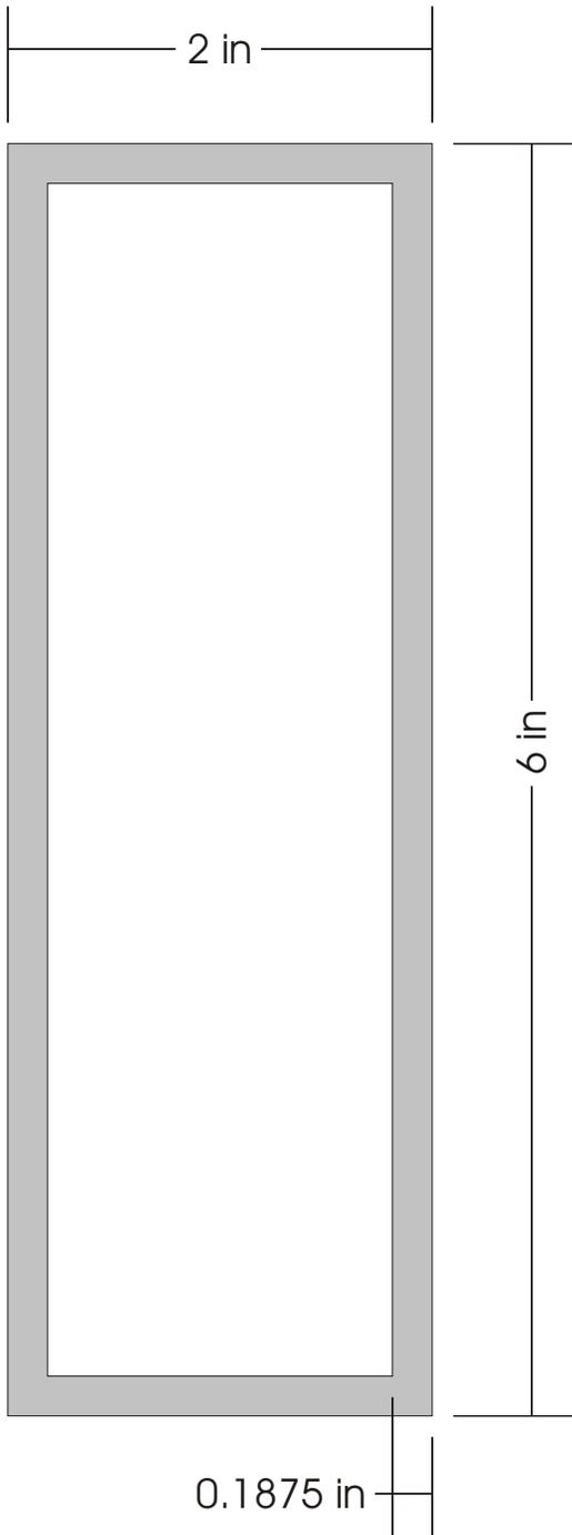
Shell is made from aluminum extrusion that is cut to length.
