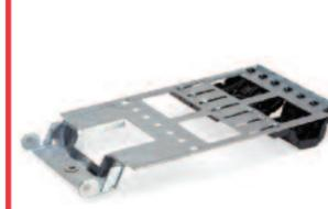
Optional drive cage with cooling fan holds four 3.5" internal disk drives. Maximum of two drive cages per system.
